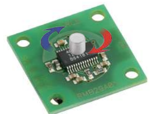
Clockwise (CW) rotation of magnet
